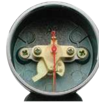
Precision-crafted, Japanese-engineered manometer movement tested to 30,000 cycles.
